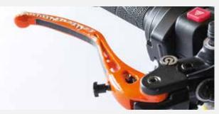
Hybrid CFRP 3D printed brake lever
