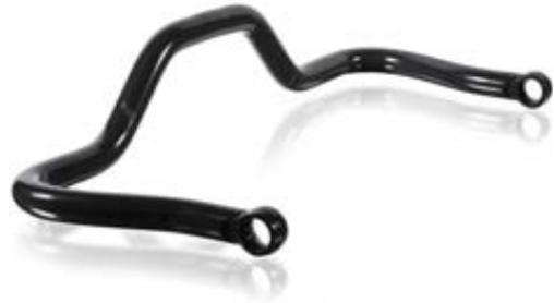
Stabilisers are among the basic components of bus and truck suspension systems because they improve vehicle stability and handling, especially when cornering. Frauenthal Automotive produces its stabilisers in Douai, France. Besides the core solid stabiliser product range, the division develops and manufactures tubular stabilisers, which are playing an increasingly important part in the weight saving technologies featured by the new generation of trucks.
