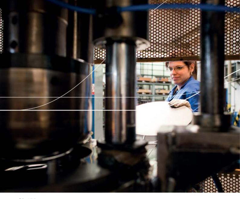
Before initiating the press process, Lucie Doležalová (33) loads blanks into the 250-tonne deep draw press by hand. The press forms a base in the sheet metal blanks, which will become air reservoirs.
