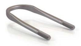
These are U-shaped mountings for leaf springs on truck axles, made at our factory in Toruń, Poland. They are critical to the safety of trucks, buses and trailers. We use state-of-the-art technologies to make them – especially in the key thread rolling, heat treatment, bending and corrosion protection coating processes.
