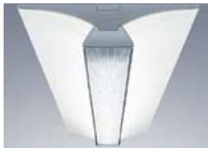
In its MELLOW LIGHT IV luminaire, ZUMTOBEL uses an innovative micro-prismatic optic. Compared to a conventional slotted sheet steel controller optic, this leads to a 20% increase in efficiency to 80%, which equates to a 16% drop in power consumption and at the same time improves the lighting quality.
