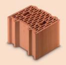
The production range of the Brenner plant includes high-quality precision-ground bricks. Wienerberger's own special bonding agent can be applied to the ground surfaces of the bricks for faster brick laying. Rows of perforations in the bricks ensure optimal thermal insulation and heat storage. The raw material is clay from the region. With saw dust added to the clay, natural, air-filled cavities are formed during the firing process. This results in improved thermal insulation.
