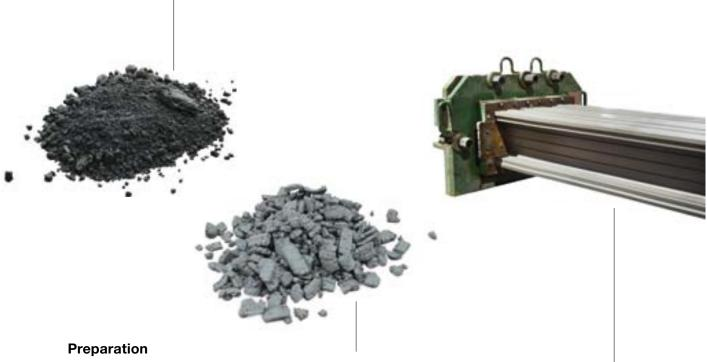
In the second step, the clay is collected from the stockpiles and transported in box feeders. It is then prepared through a grinding (pam mill) and milling process (roller mill). Water and sand – and for clay blocks, pore-forming agents like sawdust – are added and mixed to achieve the right consistency. The clay is next transported to a storage area (mud house) by conveyor belts, and from here fed through rotary disk feeders into the extruder.
