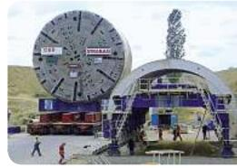
Tunnel boring machine, Perschling Tunnels, Austria
