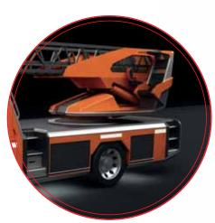
To give the operator the best possible view of the top of the ladder and the rescue cage no matter what position the ladder is in, the back and armrest of the control stand automatically tilt as much as 30 degrees to the rear.
