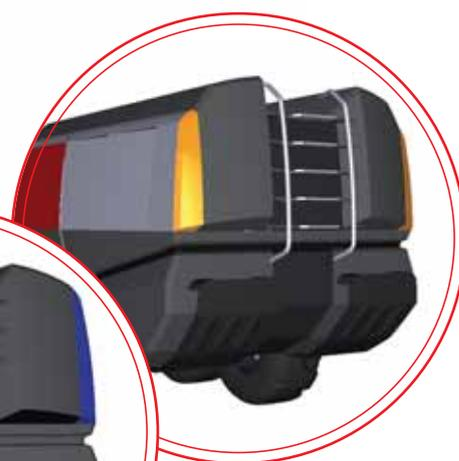
Another highlight of the development effort is the flap lids of the equipment lockers, which can now be opened pneumatically - from right beside the flap. The engine compartment and pump compartment fairings can be raised hydraulically, making for much greater ease of handling during servicing.
