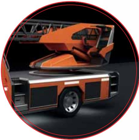
To give the operator the best possible view of the top of the ladder and the rescue cage no matter what position the ladder is in, the back and armrest of the control stand automatically tilt as much as 30 degrees to the rear.
