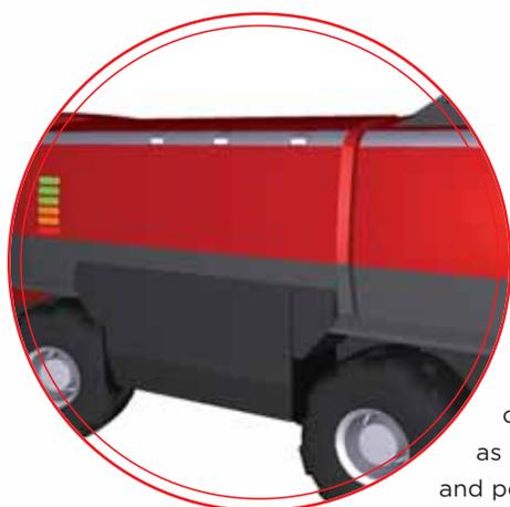
For the superstructure, only high-grade, corrosion-resistant materials are used, such as aluminium, GRP mouldings for the fairings and polypropylene for the extinguishant tank.
