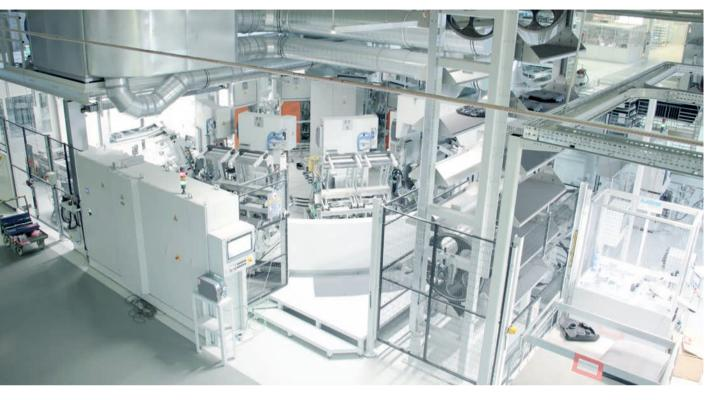
Soft engine covers are manufactured at the Hörsching location using a fully automated system, which provides short cycle times and great component flexibility.
