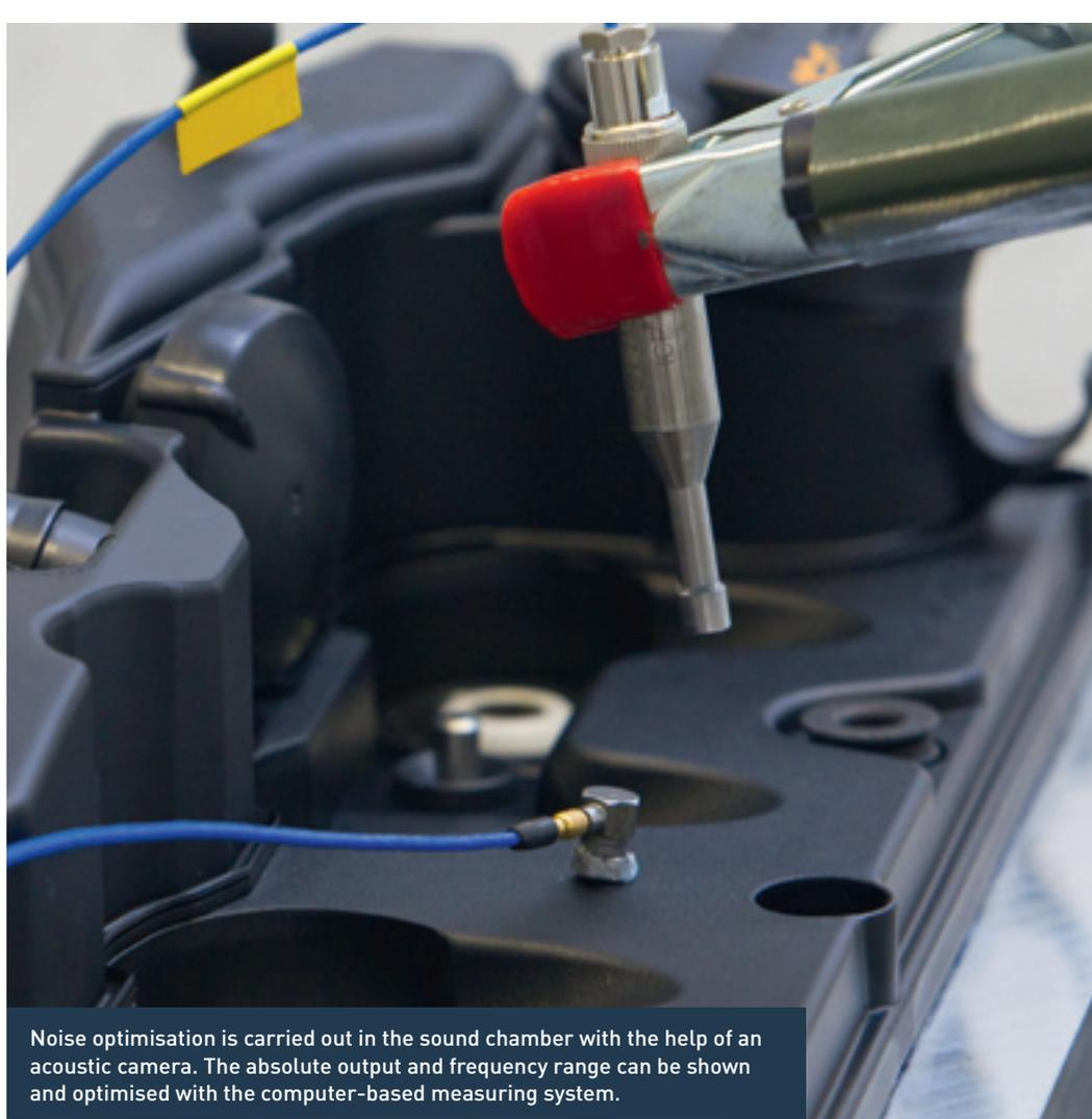
Noise optimisation is carried out in the sound chamber with the help of an acoustic camera. The absolute output and frequency range can be shown and optimised with the computer-based measuring system.
