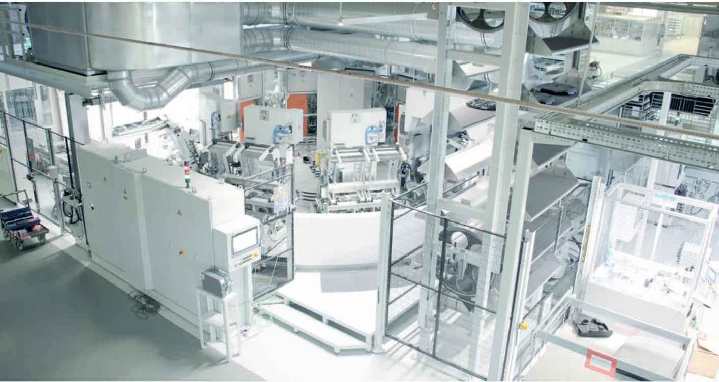
**Soft engine covers** are manufactured at the Hörsching location using a fully automated system, which provides short cycle times and great component flexibility.
