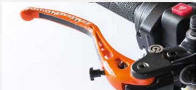
Hybrid CFRP 3D printed brake lever
