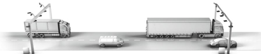
**Section Control** – Measuring the average speed over a road section is gaining in importance as a measure for improving traffic safety. Such traffic monitoring systems automatically evaluate whether vehicles are driving within legal speed limits and encourage good driving behavior. Experience has shown that monitoring the driving speed over entire road sections significantly reduces the number of road accidents while helping to improve the environmental situation.
