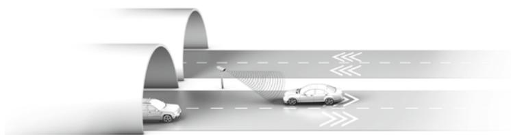
**Incident Detection System** – When accidents occur, seconds can be crucial. Fast and efficient coordination of the rescue effort is imperative for saving human lives. The Kapsch Incident Detection System uses smart video technology for reliable detection of events and hazardous situations, such as smoke, wrong-way drivers, illegally stopped vehicles or lost cargo, therefore assuring safe operation and traffic flows in tunnels and along roads.
