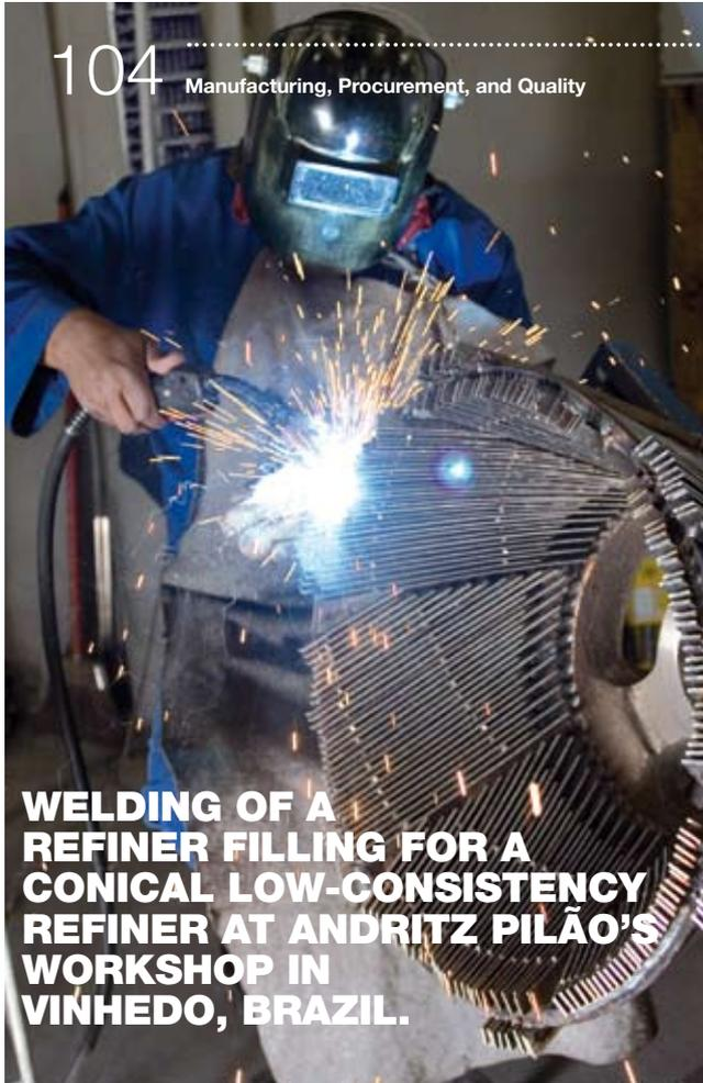
**WELDING OF A REFINER FILLING FOR A CONICAL LOW-CONSISTENCY REFINER AT ANDRITZ PILÃO'S WORKSHOP IN VINHEDO, BRAZIL.**
