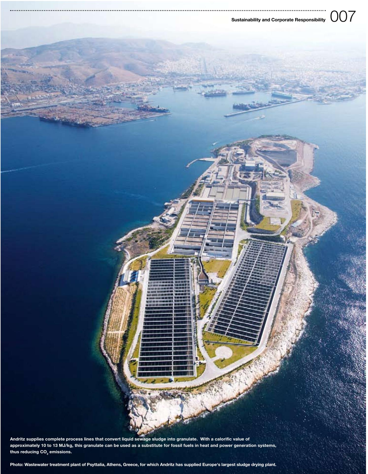
Andritz supplies complete process lines that convert liquid sewage sludge into granulate. With a calorific value of approximately 10 to 13 MJ/kg, this granulate can be used as a substitute for fossil fuels in heat and power generation systems, thus reducing CO<sub>2</sub> emissions.
