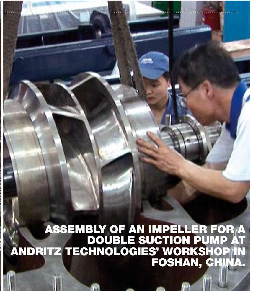
**ASSEMBLY OF AN IMPELLER FOR A DOUBLE SUCTION PUMP AT ANDRITZ TECHNOLOGIES' WORKSHOP IN FOSHAN, CHINA.**
