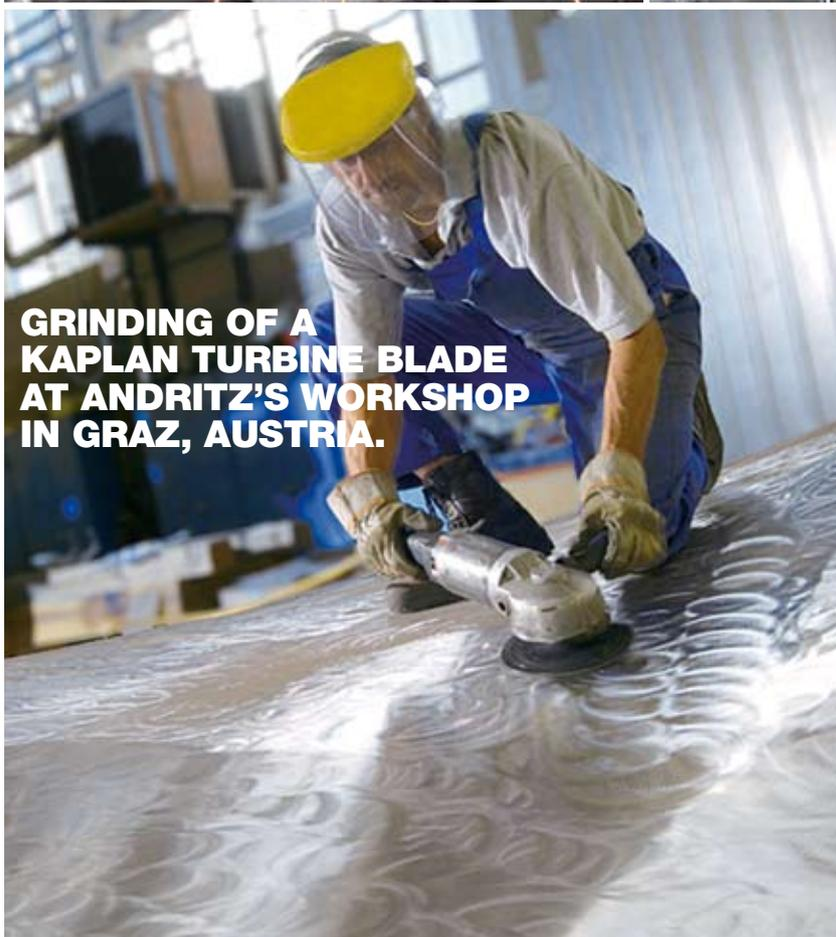
**GRINDING OF A KAPLAN TURBINE BLADE AT ANDRITZ'S WORKSHOP IN GRAZ, AUSTRIA.**
