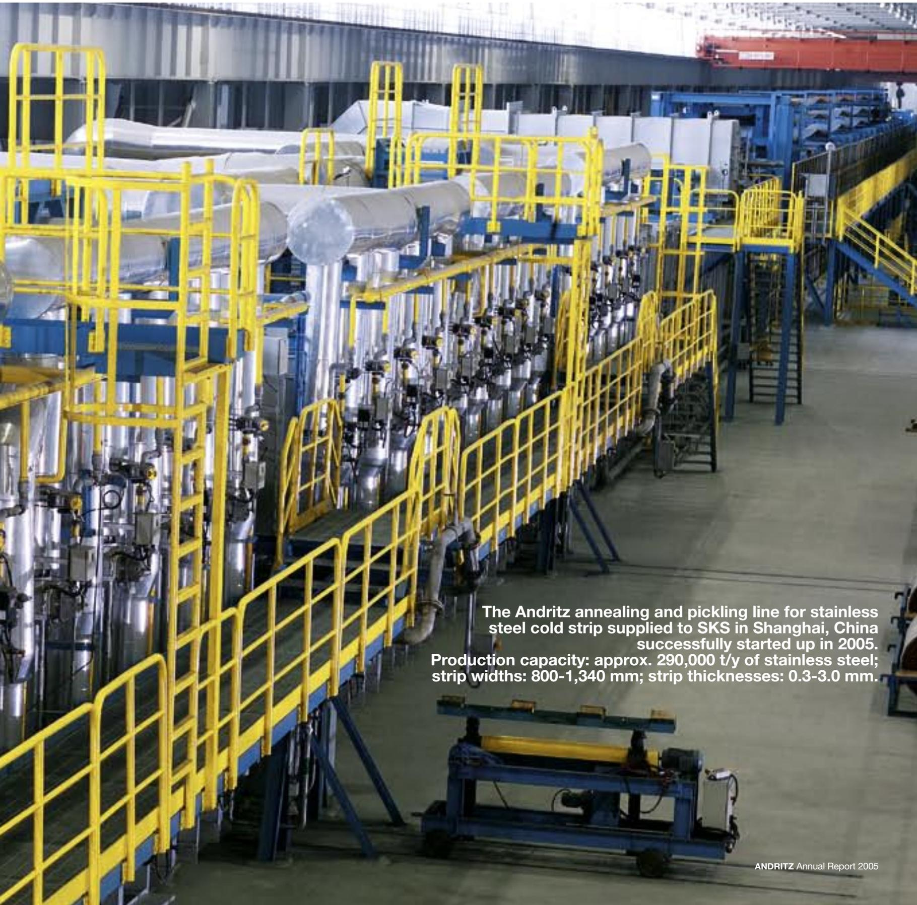
The Andritz annealing and pickling line for stainless steel cold strip supplied to SKS in Shanghai, China successfully started up in 2005. Production capacity: approx. 290,000 t/y of stainless steel; strip widths: 800-1,340 mm; strip thicknesses: 0.3-3.0 mm.
