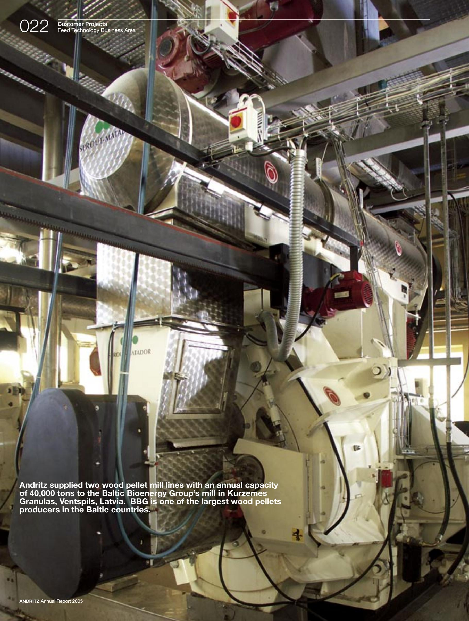
Andritz supplied two wood pellet mill lines with an annual capacity of 40,000 tons to the Baltic Bioenergy Group's mill in Kurzemes Granulas, Ventspils, Latvia. BBG is one of the largest wood pellets producers in the Baltic countries.
