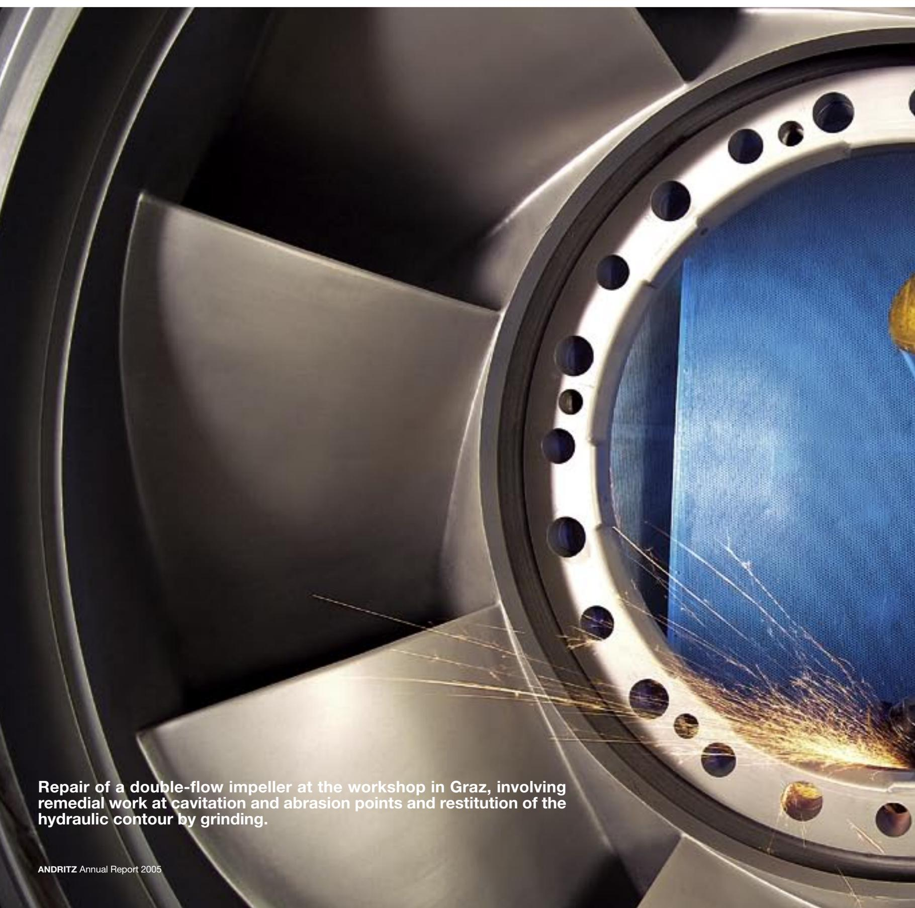
Repair of a double-flow impeller at the workshop in Graz, involving remedial work at cavitation and abrasion points and restitution of the hydraulic contour by grinding.
