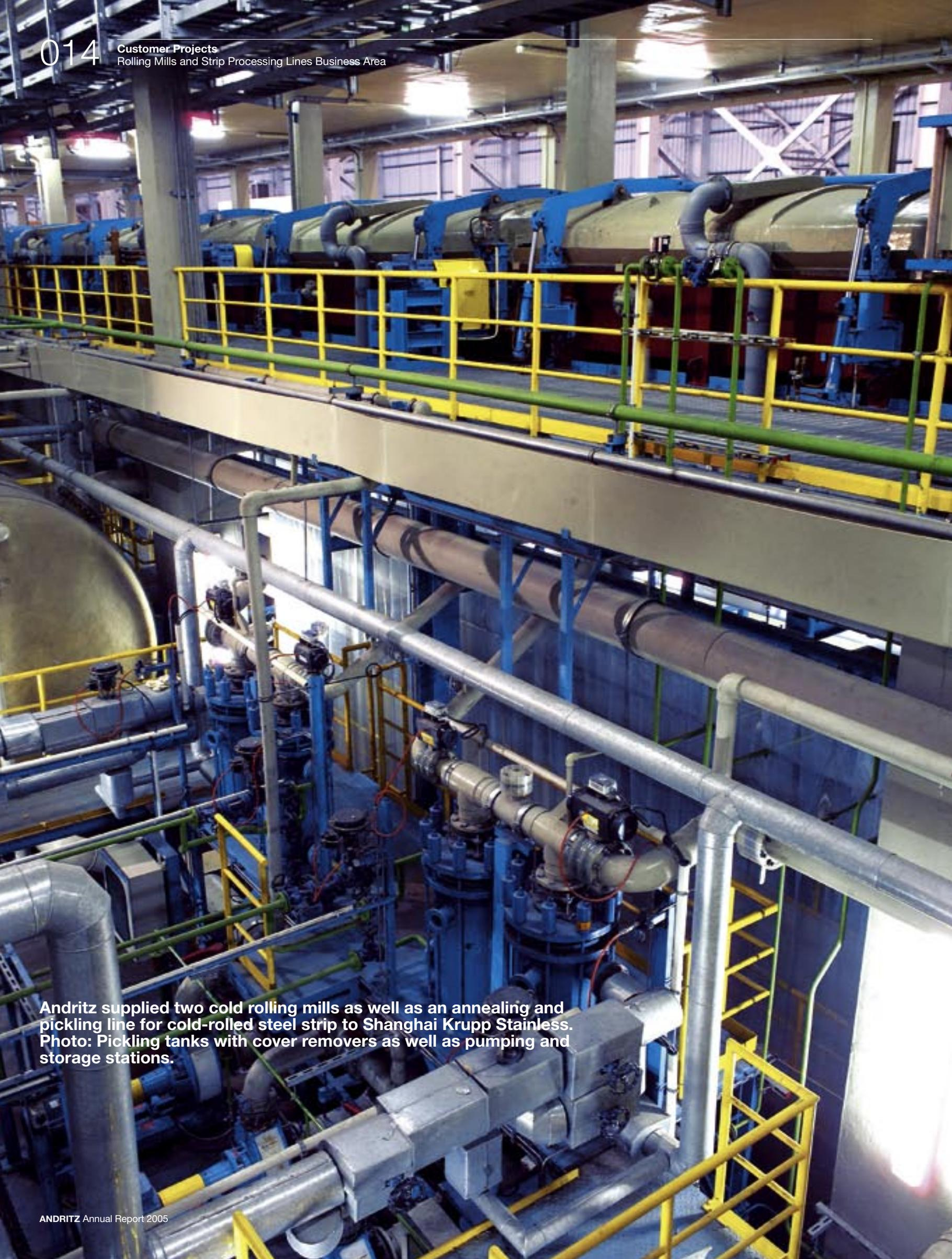
Andritz supplied two cold rolling mills as well as an annealing and pickling line for cold-rolled steel strip to Shanghai Krupp Stainless. Photo: Pickling tanks with cover removers as well as pumping and storage stations.
