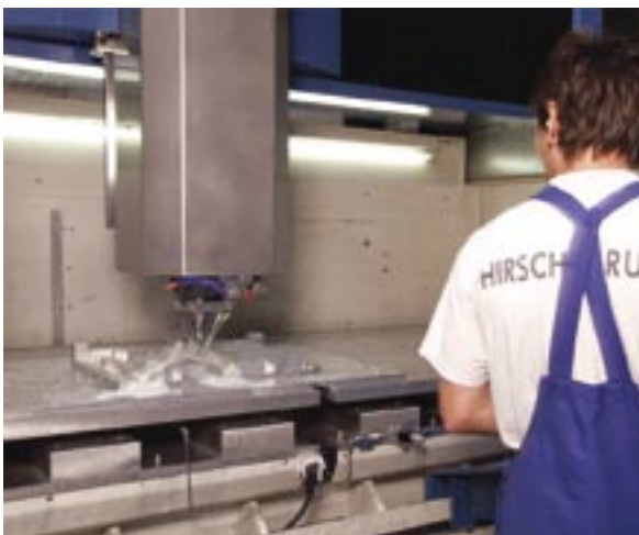
High-speed processing center for molds
