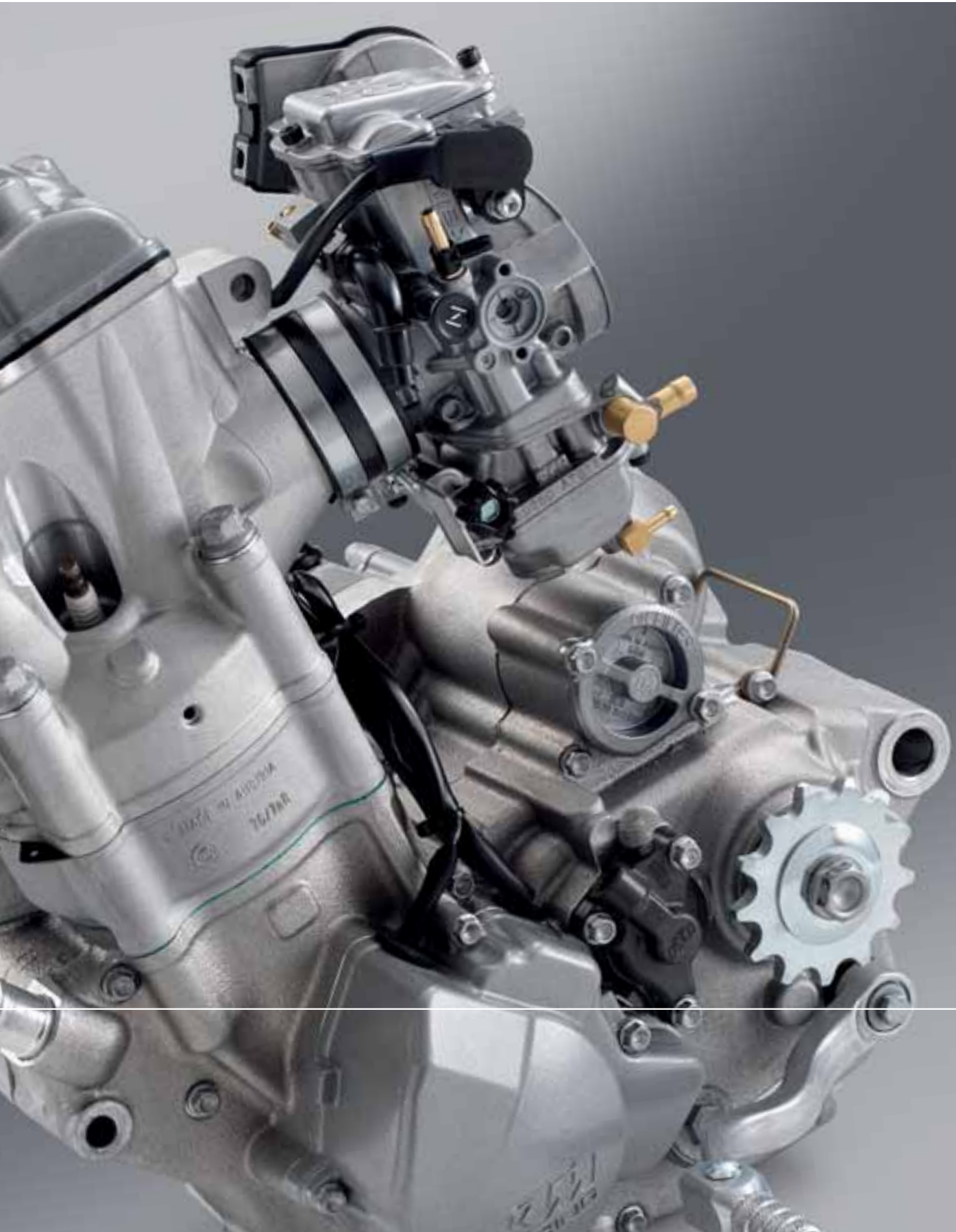
KTM Motor 250 SX-F. The KTM 250 SX-F engine.
